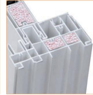
Thermally welded multi-chambered 5-5/8" main frame provides superior strength and thermal insulation. Optional foam filled insulated extrusions provide better thermal efficiency.
