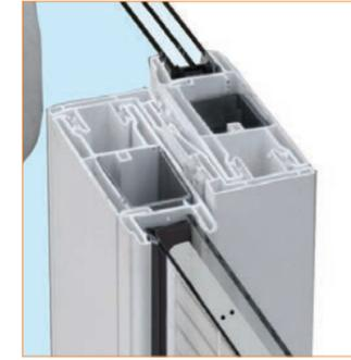
Interlocking meeting rail system with quadruple weather-stripping for controlling infiltration of air, water, dust, and noise. Full length heavy gauge reinforcements in meeting rails and pull rail provide great rigidity and strength.
